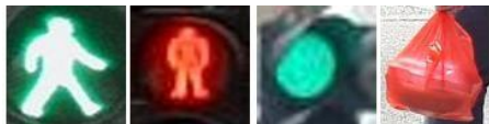
Figure 3. New images created after HSV Segmentation, binary conversion, labelling and extraction for image classification.
